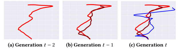
Figure 4: The key phases of the surprise search algorithm. Surprise search uses a history of two generations ( h = 2 ) and 15 clusters ( k = 15 ) in this example. The example centroid of a cluster of trajectories in this example is a trajectory depicted as a red line in generation t-2 in this example (a). The centroid trajectory of t-1 (b) and the prediction of the trajectory for generation t (c) are depicted as dark red and blue lines, respectively.
