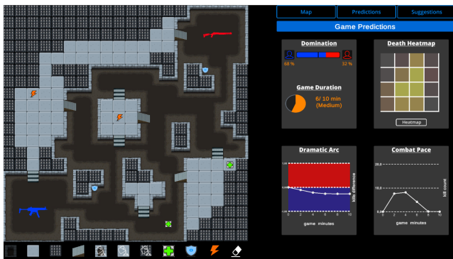
Fig. 2: SuSketch gameplay predictions: the second tab shows the predicted kill ratio of players and match duration, the heatmap of predicted death locations and the temporal progression of each player’s kill ratio and kills per 2 minutes.
